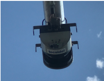
Figure 4 Overhead Laser for vehicle shape classification
