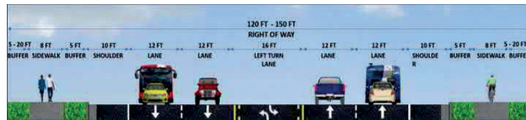
Proposed Roadway Typical Section
